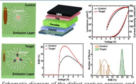
Schematic diagram of the defect capture process and performance of perovskite light-emitting diodes
